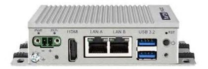
The primary purpose of the Laguna WashGuard is to act as a temporary replacement for the Main  $r \cdot TC$  in case of failure. It operates temporarily for 15 days, allowing time for the Main  $r \cdot TC$  to be repaired or replaced. The device utilizes the Main  $r \cdot TC$  software license and is limited to 15 days of car wash operation.
